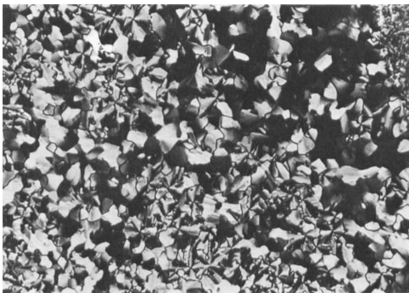
FIGURE 3 Focal conic fan texture of D , columnar phase.
